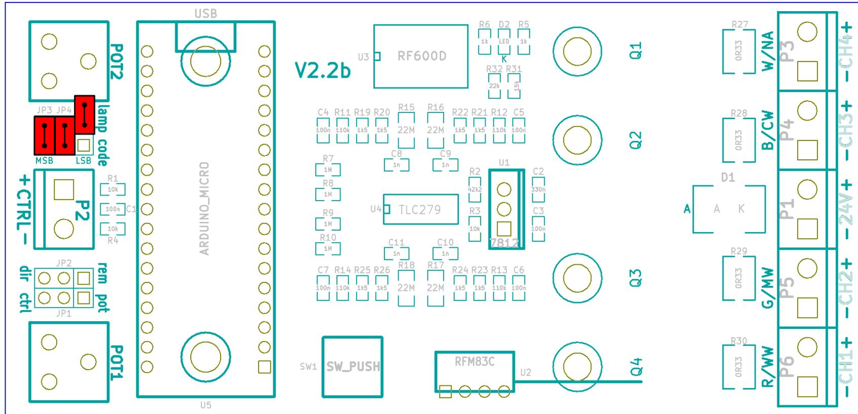
**note: JP5 does not make contact, either leave at one pin or leave out**
