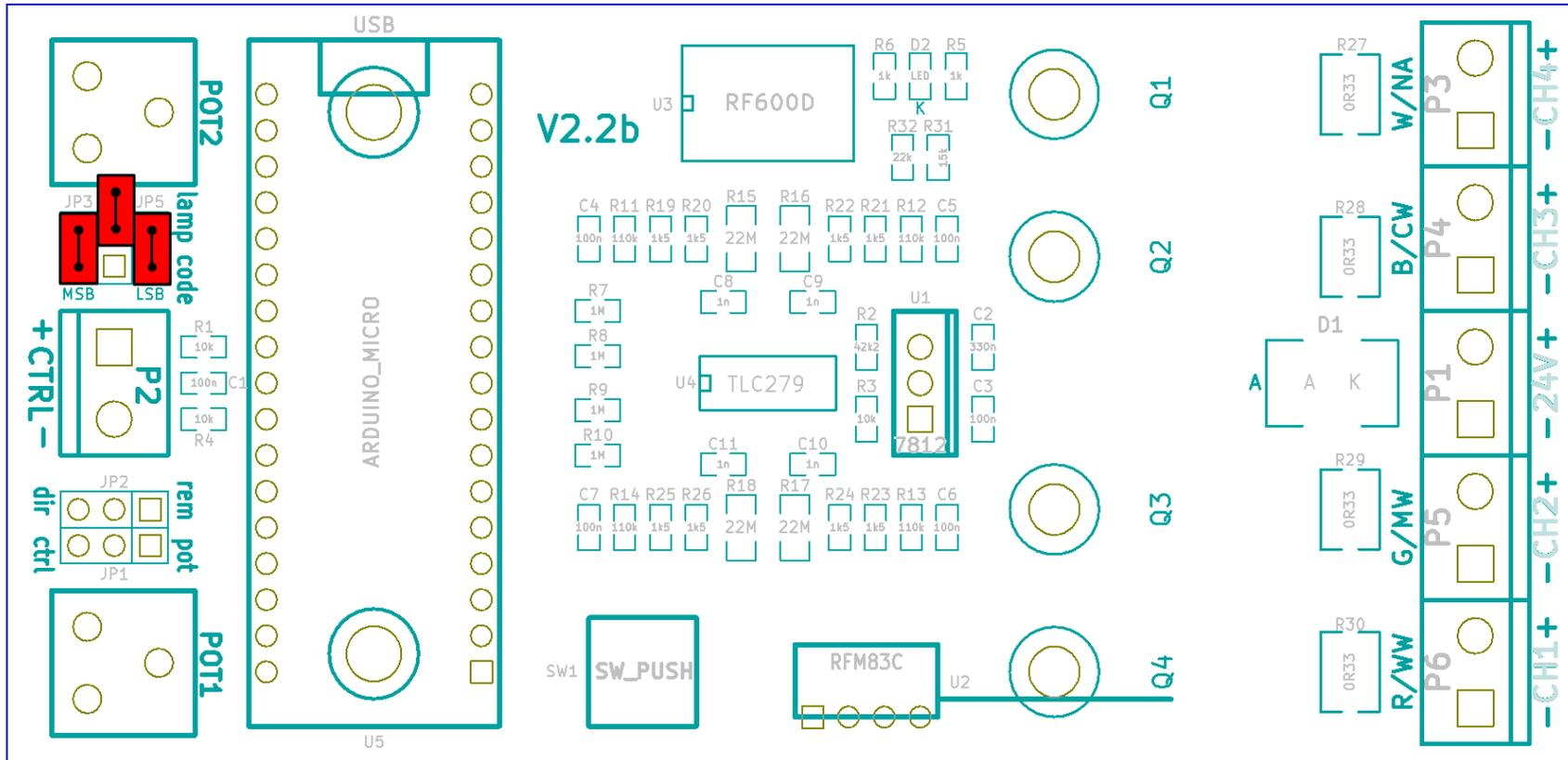
**note: JP4 does not make contact, either leave at one pin or leave out**
